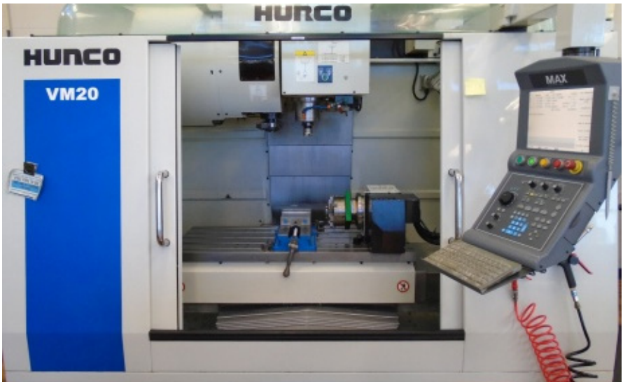
Hurco VM20: Computer operated machining center Photo credit: Anne Weitzel
